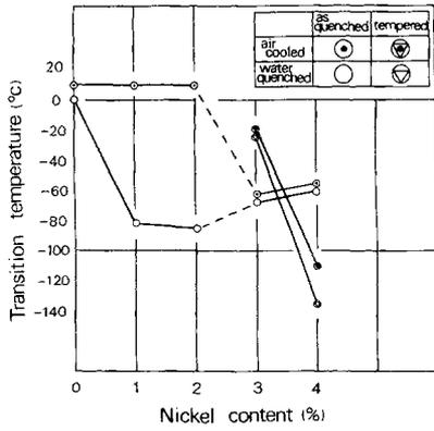
Figure 5 Effect of nickel content and heat treatment on the energy transition temperature.
