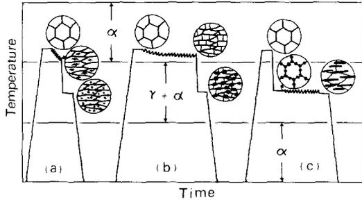
Figure 2 Schematic diagram of various precipitation states of  $\gamma$ -phase due to thermo-mechanical processing. (a) Homogeneous, (b) inhomogeneous and (c) elongated.
