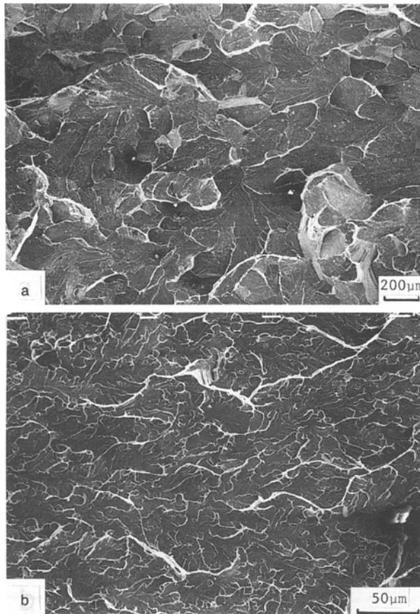
Figure 6 Scanning electron micrograph of the fracture surface. Ni = (a) 3% and (b) 4%.
