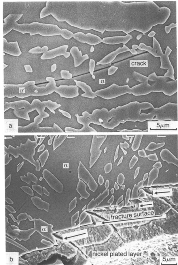
Figure 8 Scanning electron micrograph of the section of nickel plated fracture surface. Dispersed martensite particles have the effect of stopping the crack propagation. (a) Inside the fracture surface and (b) fracture surface.
