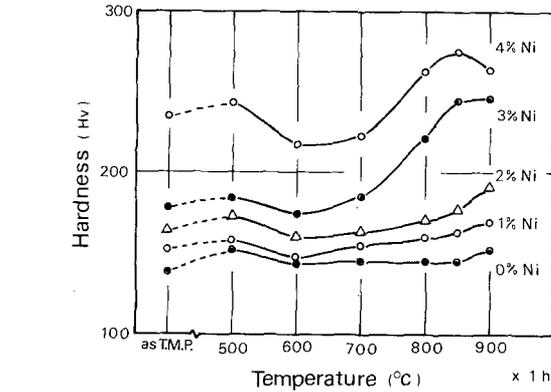
Figure 3 Vickers hardness of the thermo-mechanical processed specimens after quenching from reheated temperatures.
