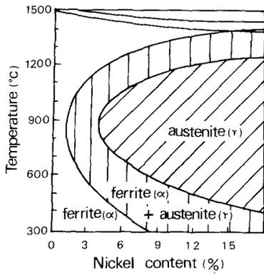
Figure 1 Fe-18Cr phase diagram containing nickel elements [10].
